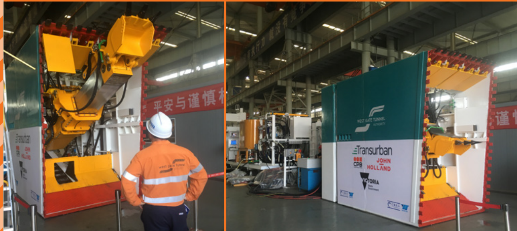
Front view (left) and side view (right) of box jacking machine.
